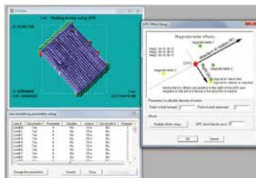
Correcting GPS Data for Offsets
