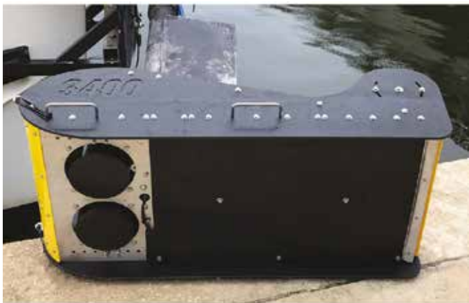
4. Large Multi-Channel Hydrophone can be configured in "Pipe Line Finder Mode"
