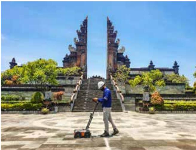
Locating and marking underground utilities in real-time in the field has been a powerful application of ground penetrating radar (GPR) for many years. A knowledgeable utility locator with a GPR system as part of their tool box is able to accurately identify buried utilities.
