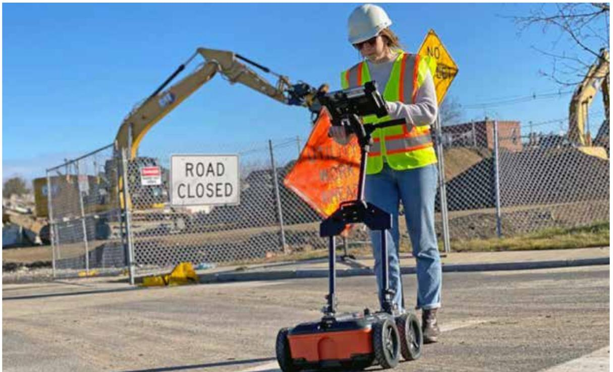
**UtilityScan is built for the utility locating professional to accelerate workflow from target detection to reporting.**
