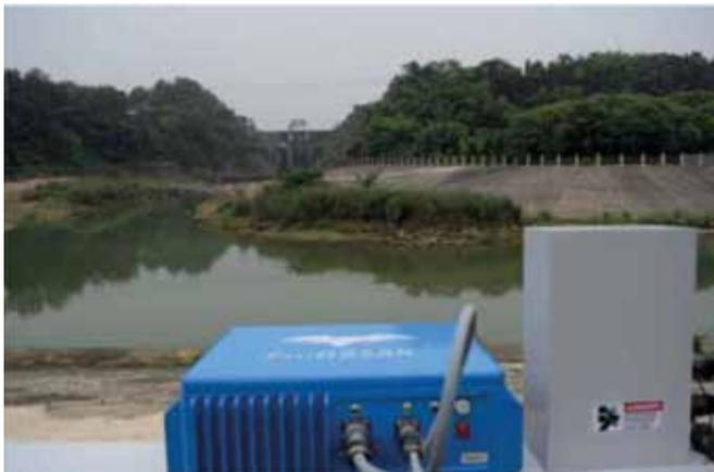
Deployment site for the FastGBSAR, about 400 meters in front of the dam.
