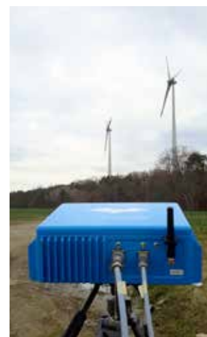
FastGBSAR installation for monitoring wind turbines.
